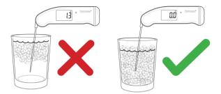
\*\* An improperly made ice bath can be off at the ice point by as much as 8 °C. See above illustration.
